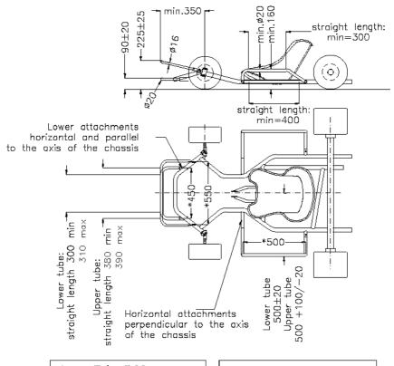
Lower Tube Ø 20mm with one constant radius.
