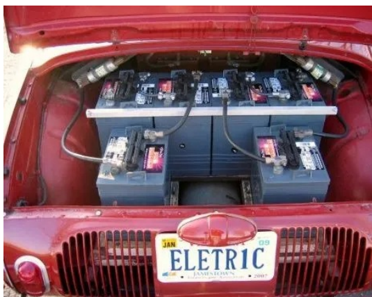
Rear-mounted batteries of a 1960 model
