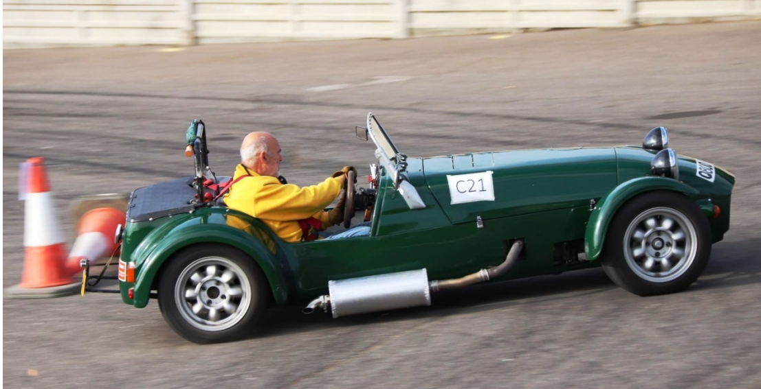
Nick's Westfield with extra wrapping of his silencer for insulation of noise and heat
